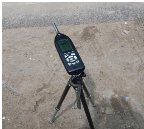
Figure.2. Sound Level Meter (Larson & Davis 831) used for noise monitoring
