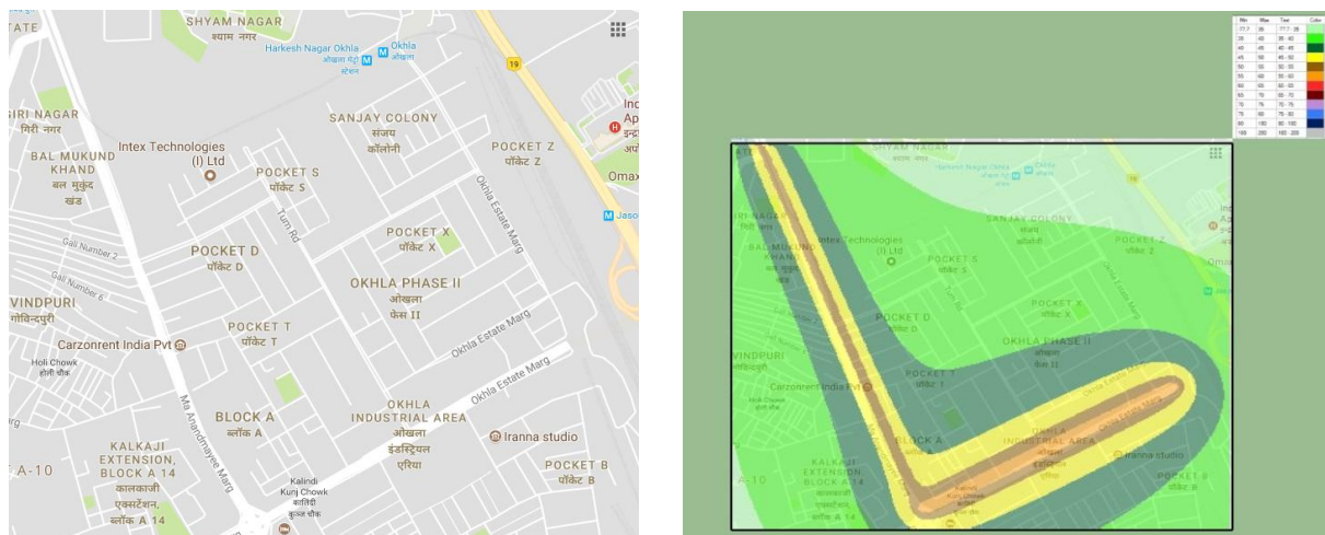
Figure.8. 2D noise mapping of industrial area phase-II
