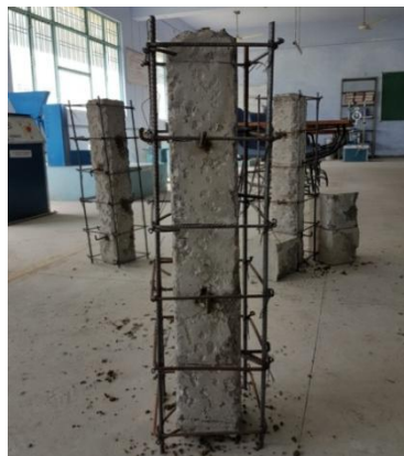
Figure No. 3 (Re-baring)
