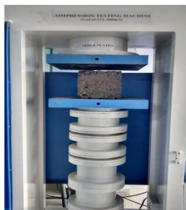
Figure No. 2 (Compression of testing Machine)
