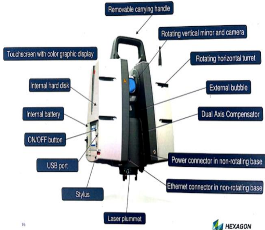
Figure 4: Components of Leica TLS Scan Station P40
