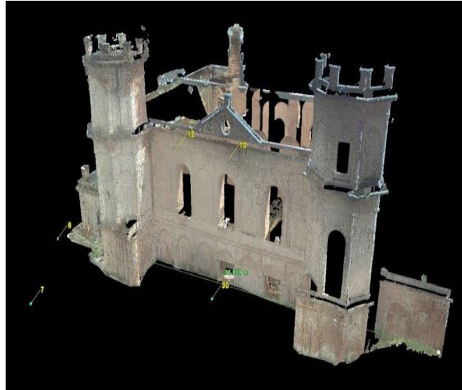
Figure 2 Point Cloud Data of Alambagh Gate with the location of TLS scanner points (after classification).
