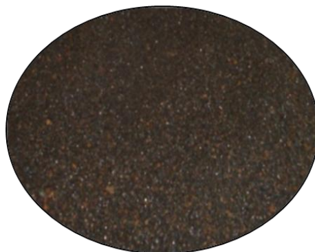
Figure 2.1 Copper Slag Particles
