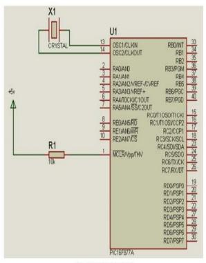
Figure 10. PIC16F877Acircuit.
