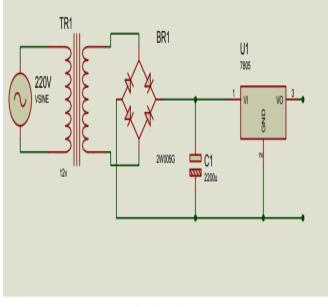
Figure 5. Powersupplycircuit.
