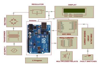
Fig. 1. Underground cable fault distance locator block diagram
