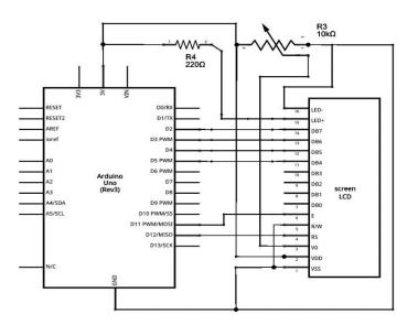
Fig.5. Circuit diagram of interconnection of LCD display with Arduino
