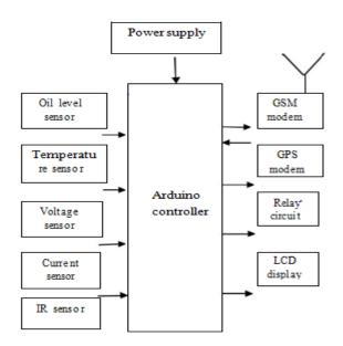
Fig.2. Block diagram of transformer monitoring and protection with GSM technology.
