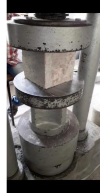
Fig-2 Shows testing of Cubes for Compressive Strength
