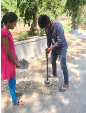
Fig-1 Shows making of Fine aggregates from Ceramic Waste.
