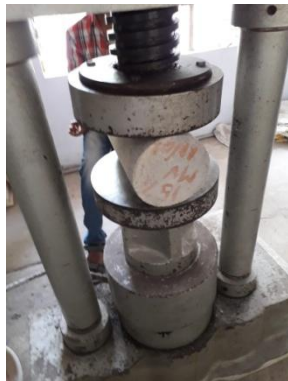
Fig-3 Shows testing of Cylinders for Split Tensile Strength
