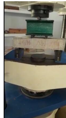
Fig-4 Shows testing of Prisms for Flexural strength
