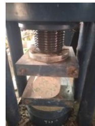
Fig.4: Split tensile Strength test
