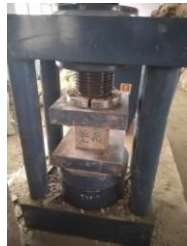
Fig.3: Compressive Strength test.
