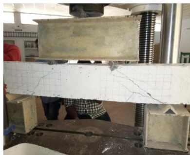
Fig 2. Shear failure of specimen
