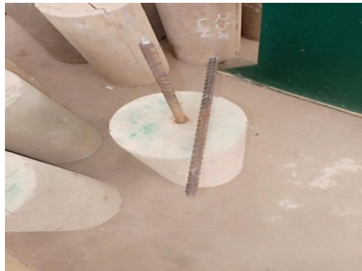
Fig.6: Failure in Steel Reinforcement for 30cm Embedded Length of Bar.
