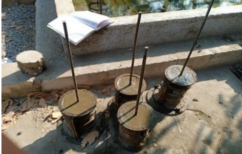
Fig.2: Casting of Cylinders.
