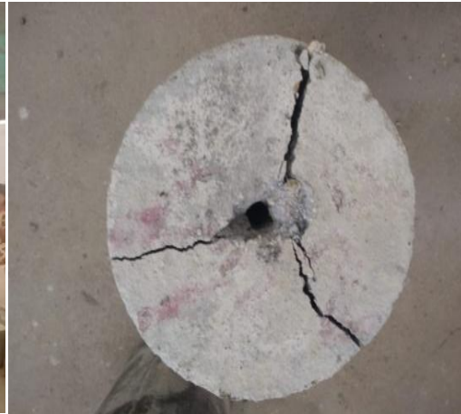
Fig.5: Splitting in Concrete for 20cm Embedded Length of Bar.
