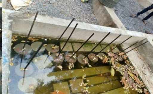
Fig.3: Specimens are in a Curing Tank.
