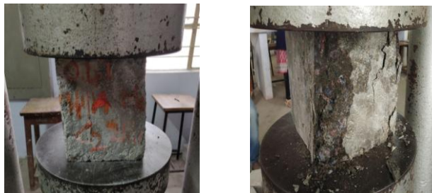
Figure -7 Compressive strength test of Cubes under ultimate load
