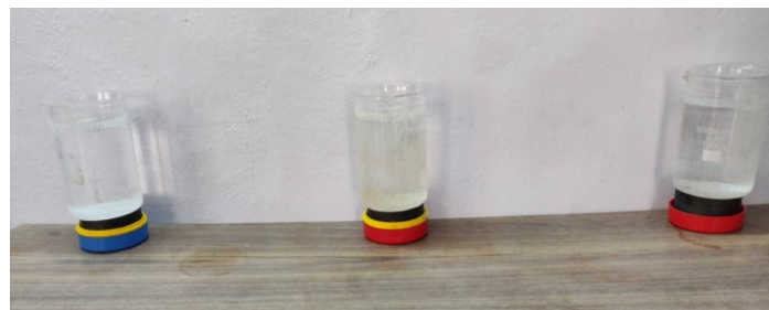
Figure-1 Showing the preparation of magnetic field treated water
