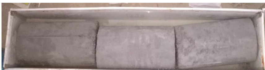
Figure -5 Curing in magnetic water with intensity of 0.6T
