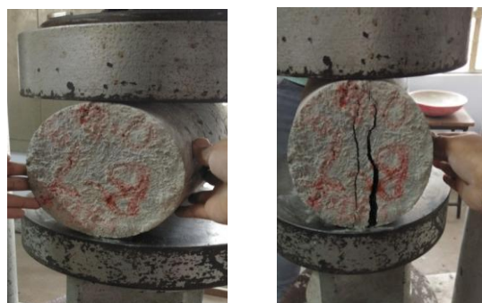
Figure -8 Split tensile test of Cylinders under ultimate load
