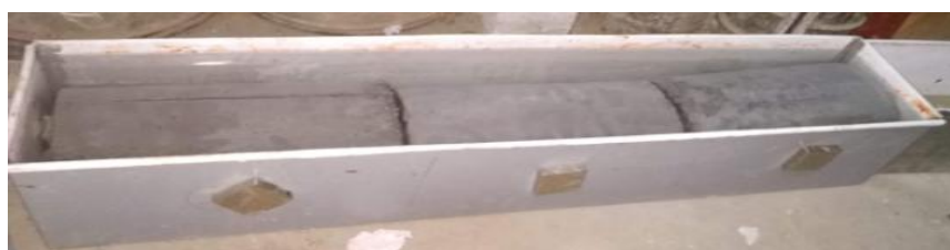
Figure -6 Curing in constant magnetic field of 0.6T
