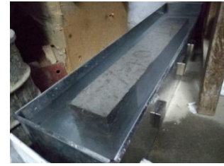
Fig 2(c) curing of beam in with magnetic structured water
