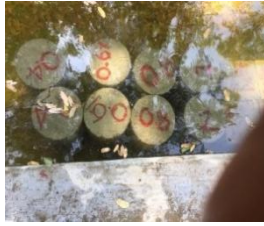
Fig 2 (a) Curing of test specimens in potable water
