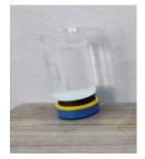
Fig. 2 Beaker placed over the magnets for magnetizing the water
