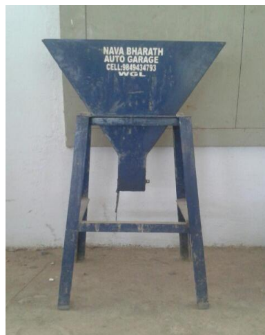
Fig. 3: V-Funnel test equipment.
