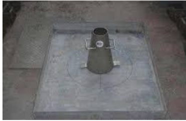
Fig. 1: Slump flow test equipment. 500R
