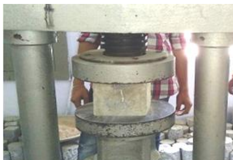
Fig 10:Compressive strength test on cube specimen
