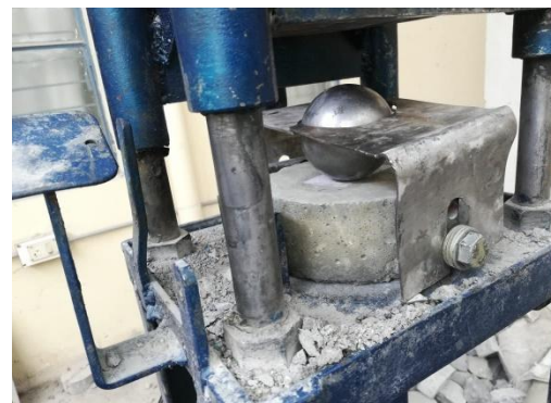
Fig.2: Steel ball placing at center of specimen
