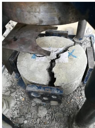
Fig 3: Failure of specimen (M35)
