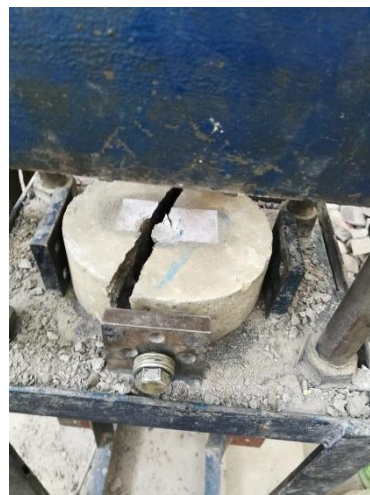
Fig 4: Failure of specimen (M45)
