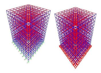
Fig:6 Building Models with fixed base and with SSI case (Martin et al (2017)).
