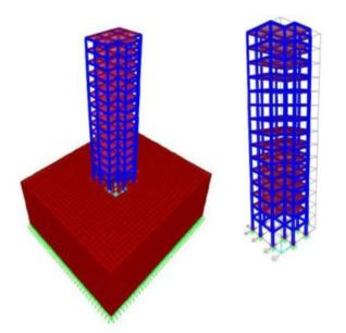
Fig.1 Shows model with fixed base with SSI and fixed base without considering SSI. (Nirav et al. 2016)
