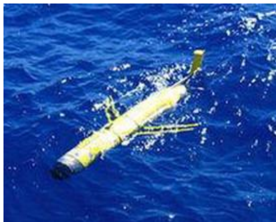
Fig 9. A Slocum glider operated by Rutgers University, U.S.A.
