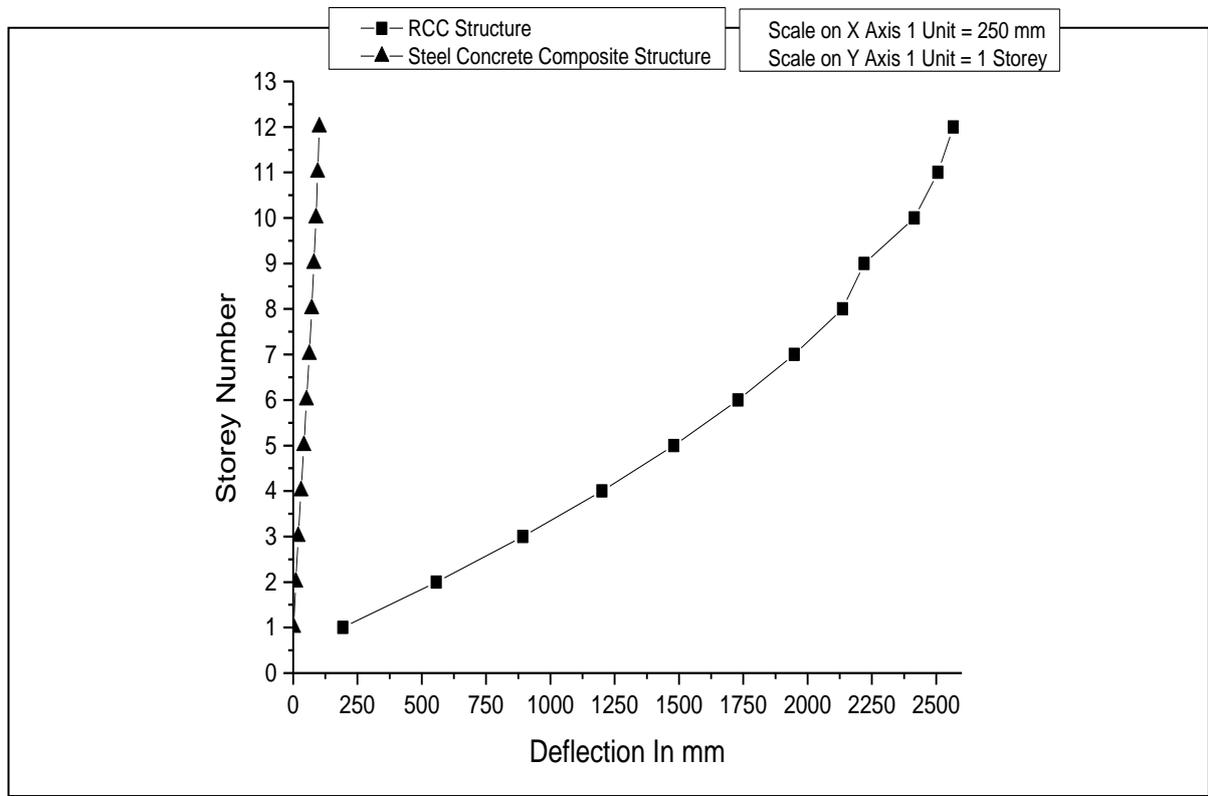
Graph 2. Comparative graph of BC sections of Steel Concrete Composite Structure and RCC Structure
