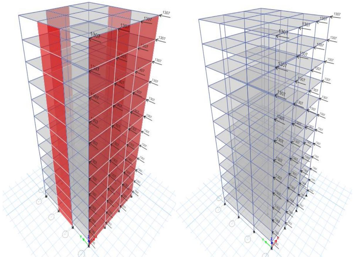
**Fig. 4.** Blast load application on beam column joints of Steel concrete composite structure and RCC structure.
