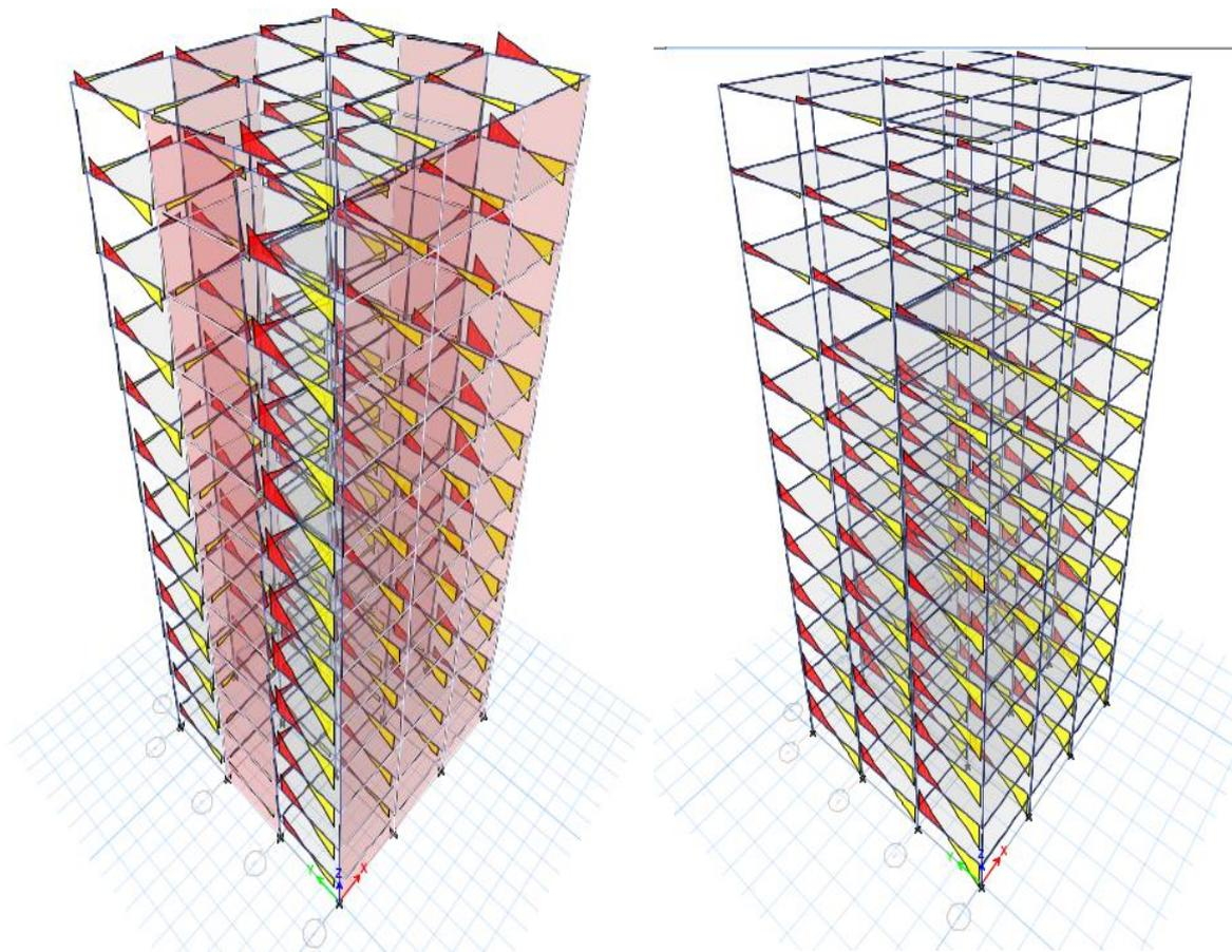
**Fig. 6.** Bending moment diagram of Steel concrete composite structure and RCC structure.
