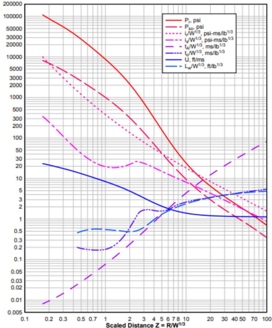
Fig 1 Free blast wave curves
