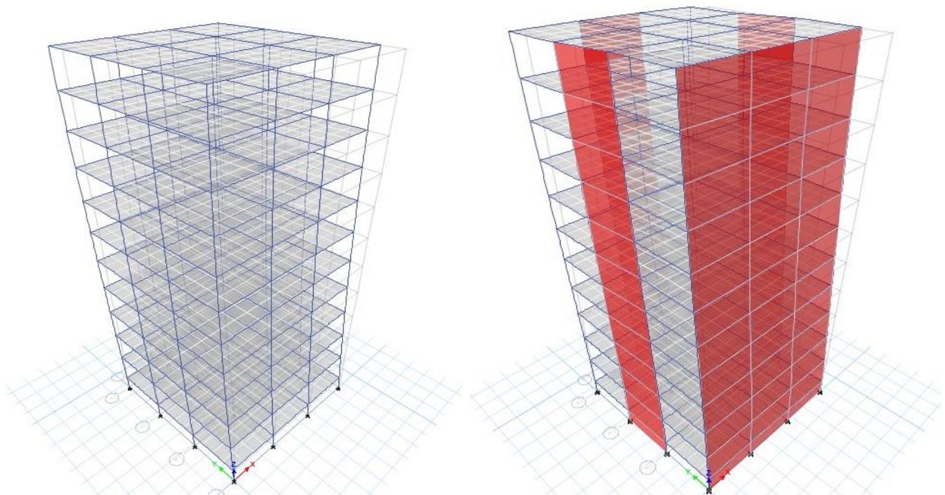
**Fig.7** Deflected shape of Steel concrete composite structure and RCC structure after application of blast load.
