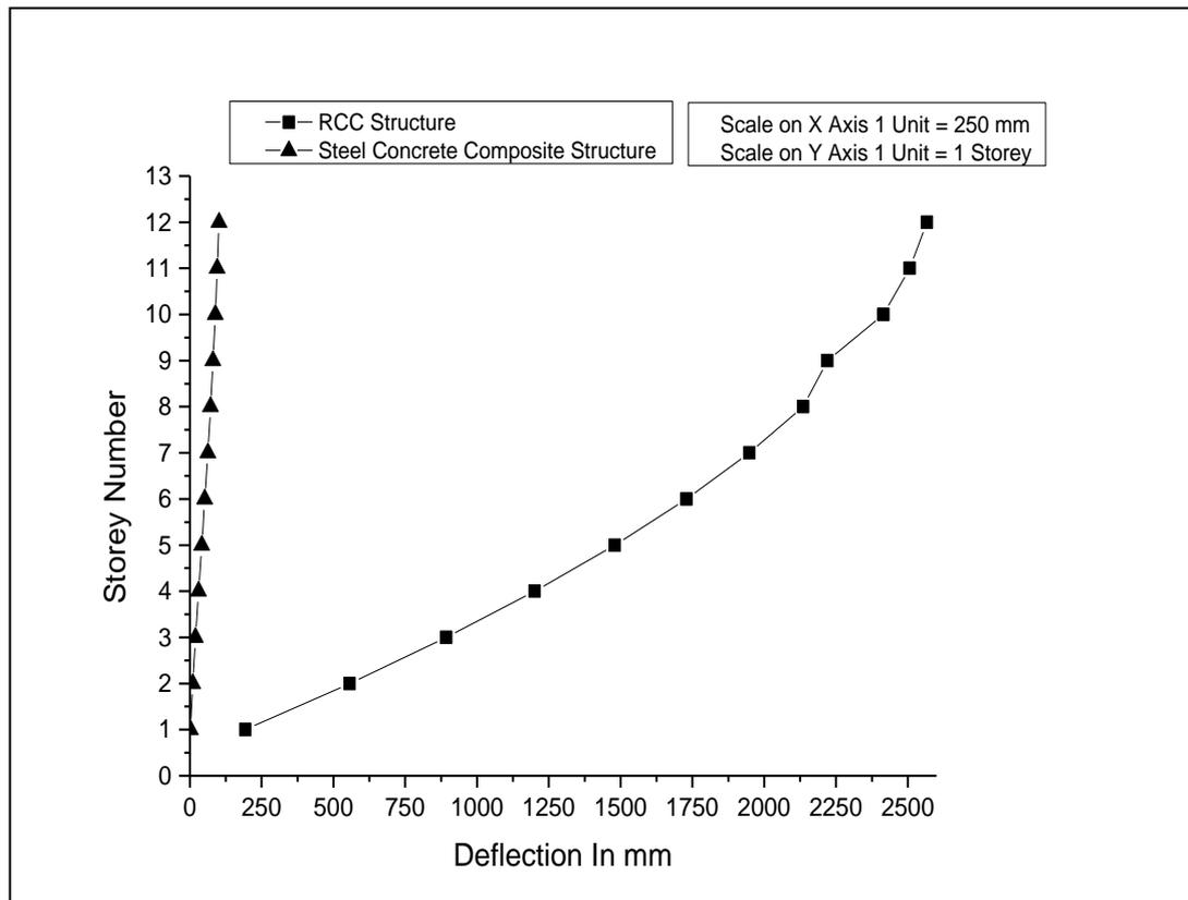
Graph 1. Comparative graph of AD sections of Steel Concrete Composite Structure and RCC Structure
