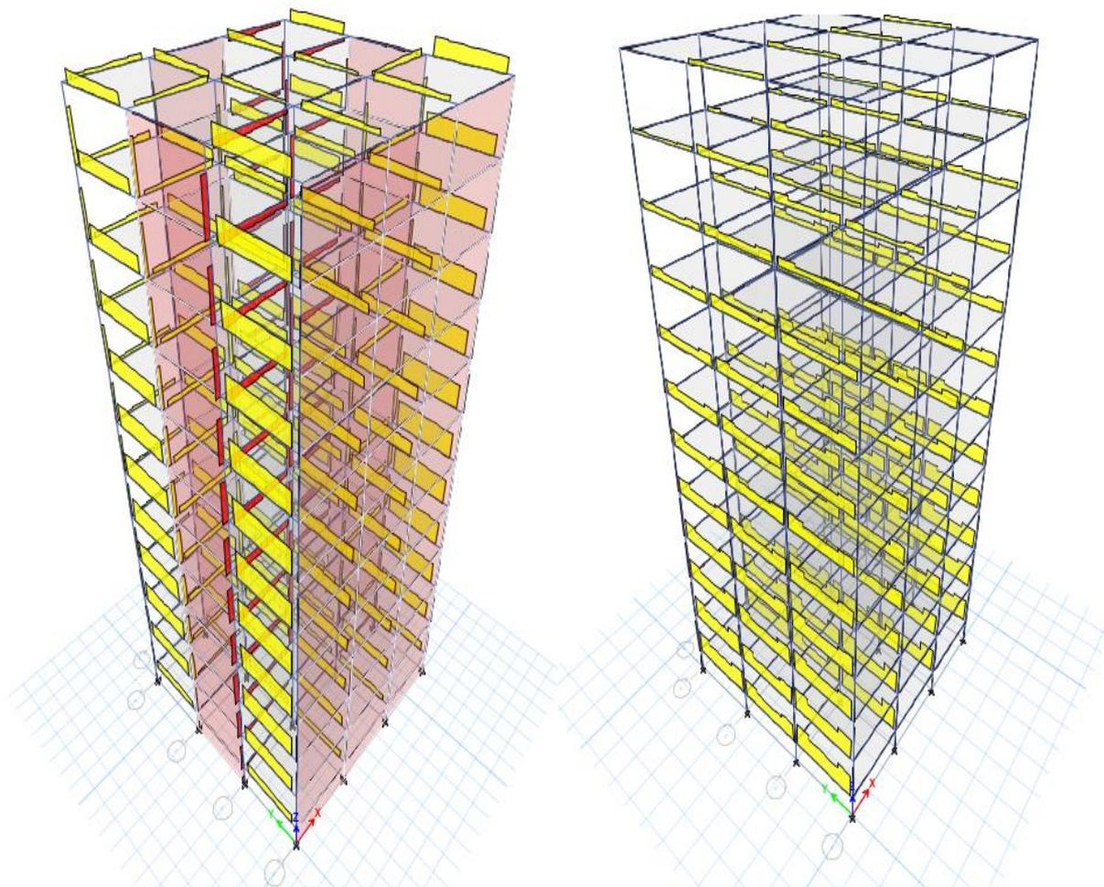
**Fig 5.** Shear force diagram of Steel concrete composite structure and RCC structure.
