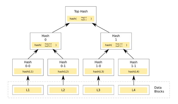
Fig 4 Block diagram of Git.Merkle trees
