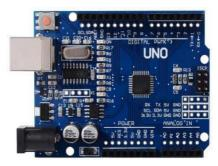
Fig: 1 Arduino UNO Board
