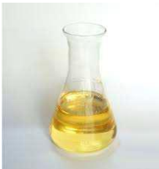
Fig 3: POE oil before mixing with SiO 2
