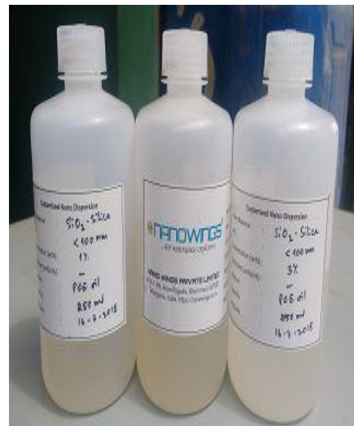
Fig 6: Nano lubricants of SiO 2
