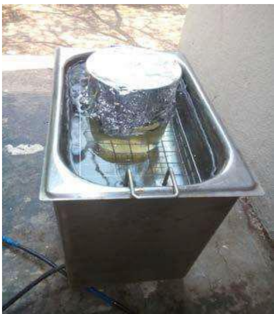
Fig 5: Stirring in ultrasonic vibrator
