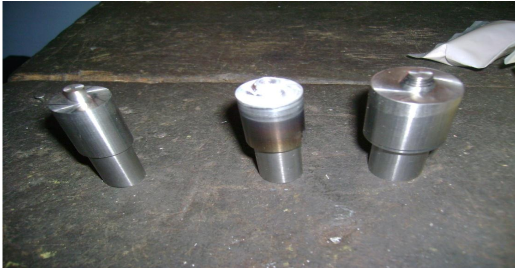
Figure 04 Tools used for friction stir welding process
