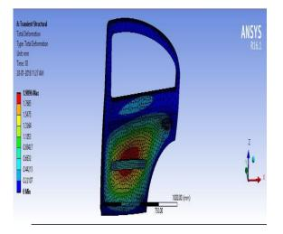
(Fig-11 Total Deformation on Aluminum Alloy-Box)
