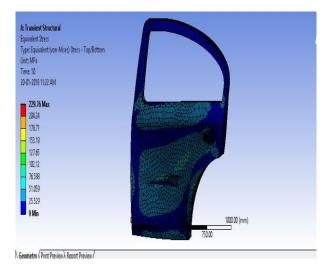
(Fig-10 Von Mises Stress Distribution of E-Glass)
