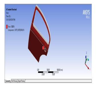
(Fig-6: load acting on outer body)
