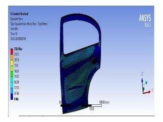
(Fig-18 Von Mises Stress Distribution on E-Glass Epoxy-C)
