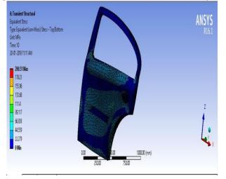
(Fig-9 Von Mises Stress Distribution of S-Glass)
