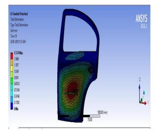
(Fig-12 Total Deformation of e-glass -box)
