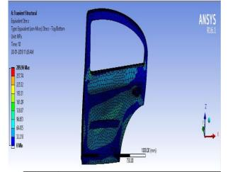
(Fig-8 Von Mises Stress Distribution of aluminum alloy -box)
