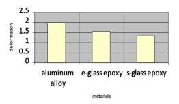
(Fig-21 Bar Chart of Deformation observed in mm box section)
