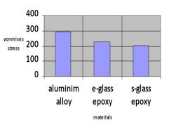
(Fig-20 Bar Chart of Von Mises Stress observed in MPa box section)
