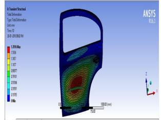
(Fig-15 Total Deformation of e-glass - c)
