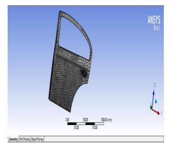
(Fig-5: Meshed model of Car door)
