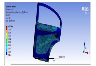
(Fig-19 Von Mises Stress Distribution on S-Glass Epoxy-C)
