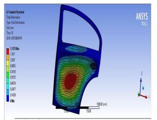
(Fig-16 total deformation of s-glass-c)
