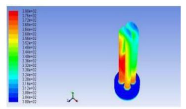
Fig.6 Temperature contour of a tube surface without fin
