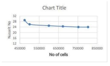
Fig. 3 Grid independency test
