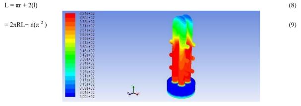
Fig.6 Temperature contour of a tube surface with fin Surface area of fin A
