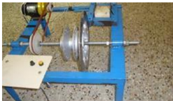
Fig.7 Assembled View of the Electro Magnetic Braking
