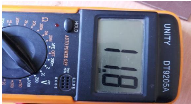
Figure 5. Input Voltage Measured from the module
