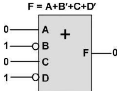
Fig. 1. Single-term function with activating input pattern.
