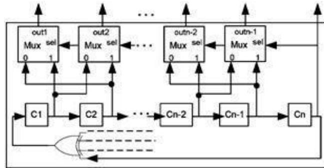
Fig. 2. BS-LFSR can be used to generate exhaustive patterns for test-per-clock BIST.
