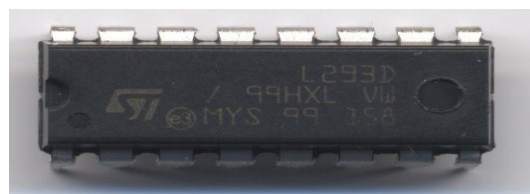
Figure 1: L293D DC Motor Driver IC
