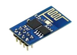
The wifi module is used to store and view data in the cloud. It is used to make simple TCP/IP connections. It contains 1MB of flash memory.
