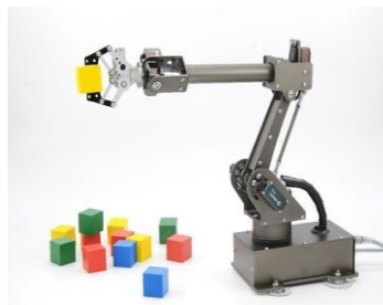
Figure 1. (a) Low cost robot using servos
