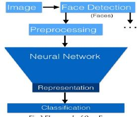
Fig 3.Flow graph of OpenFace
