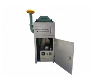
The APM 460 NL uses an IMPORTED brushless, continuous rated induction motor driven blower to significantly reduce equipment downtime, maintenance efforts and inconvenience to community. This new improved PM 10 sampler avoids problems arising due to frequent brush wear and limited armature life of blowers used in earlier models.
