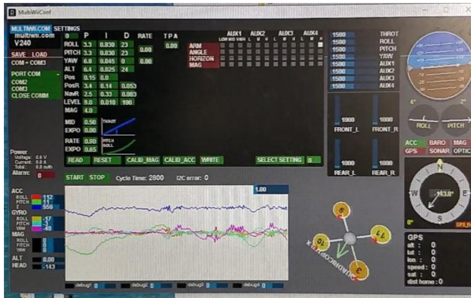
Fig.6. Gyroscope and Accelerometer calibration using MultiWiiConf application.
