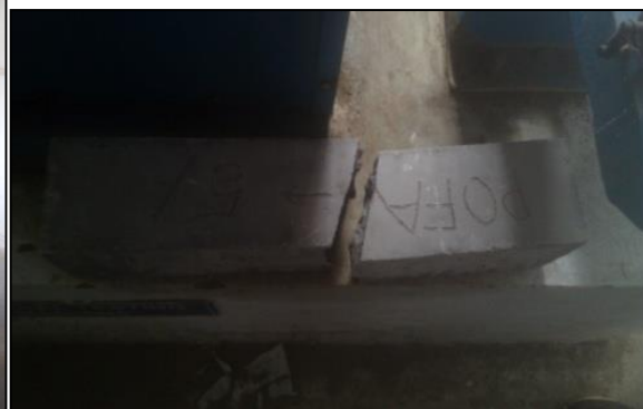
Fig.12 prism failure after testing
