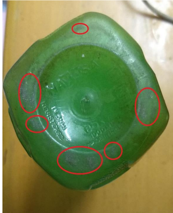
Fig. 2.: Bottom part of bottle with regions of dirt marked in red
