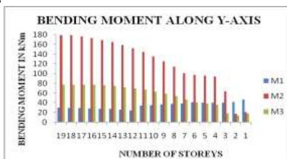
Fig.7 Bending moment along Y-axis in kNm
