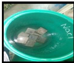
Fig.6 Cubes in Chloride solution
