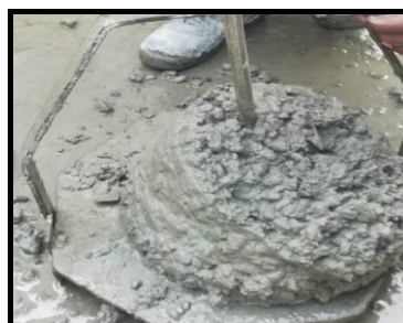
Figure.3 Slump Cone Test for Workability of GPC
