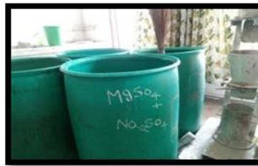
Fig.5 Cubes in Sulphate attack test
