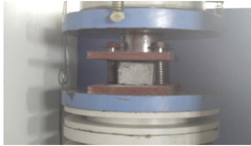
Figure - Test set-up for compressive strength test
