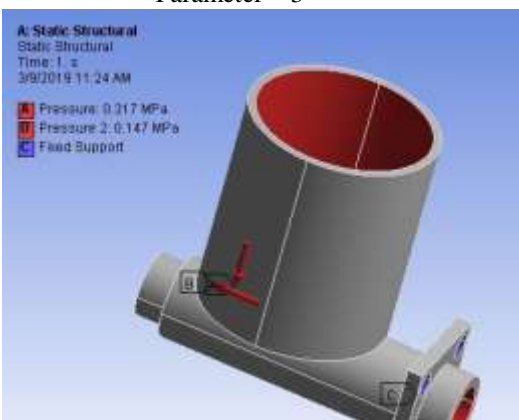
Fig 5.59 structural analysis at a pressure of 0.317 Mpa
