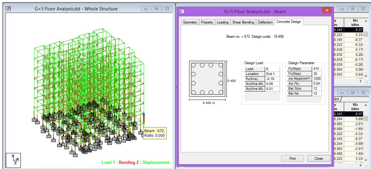
**Fig. 13** Column 672 Reinforcement
