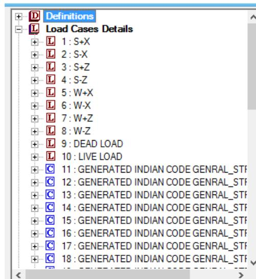
Fig. 8 Load applied in STAAD.Pro
