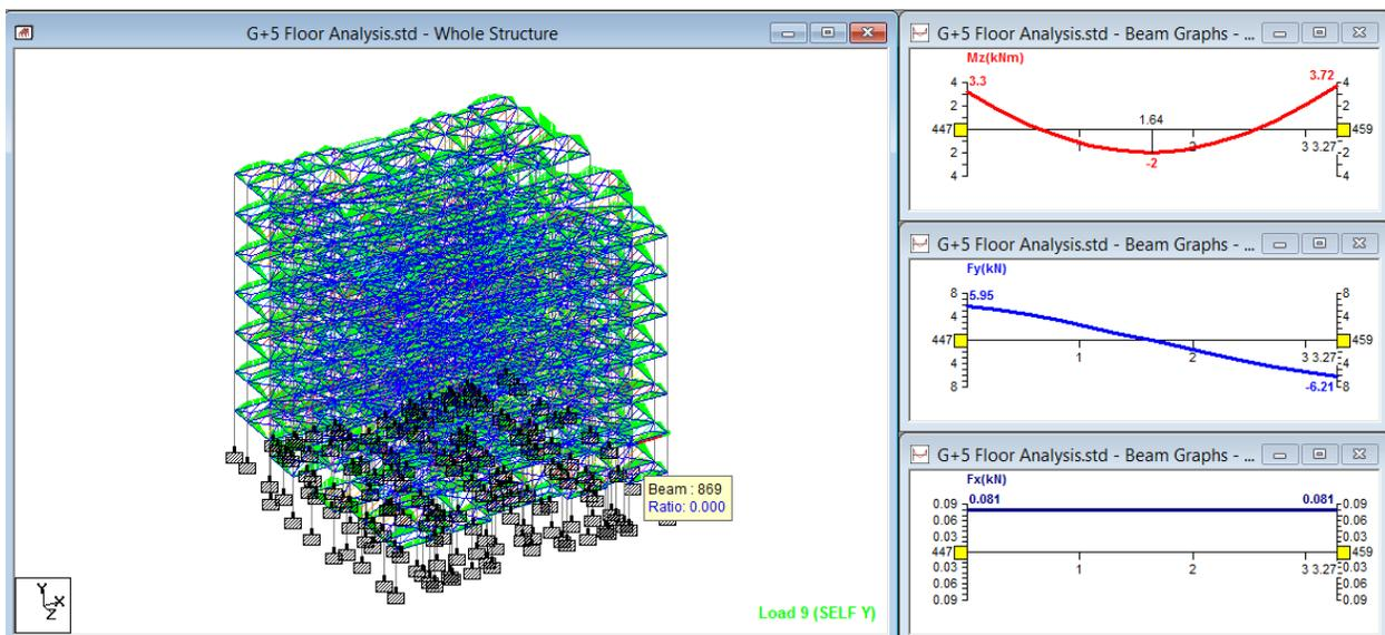
**Fig. 11** Beam bending moment shear force and axial force diagram
