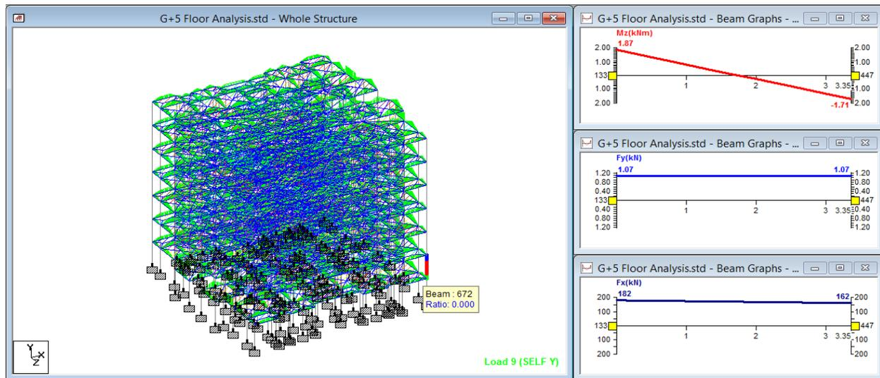
**Fig. 14** Beam bending moment shear force and axial force diagram of Column No. 672
