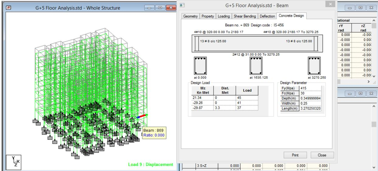
**Fig. 10** Beam 869 Reinforcement
