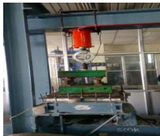
Plate 9: Testing of slab for flexural strength
