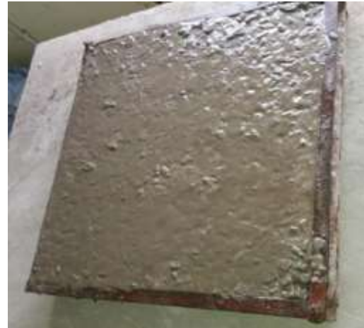
plate 7: Slab mould filled with concrete
