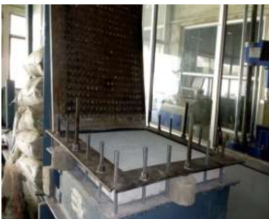
Plate 8: Slab testing frame with fixed ends
