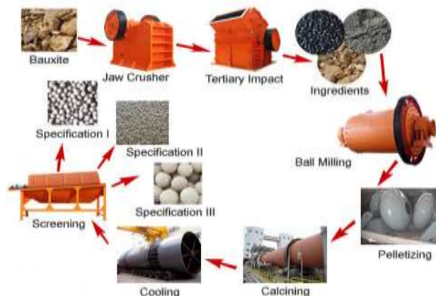
Plate 4: Flow chart of LECA Manufacturing process
