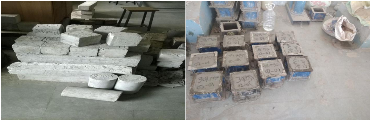
Fig 2.3 casting of cubes and cylinder
