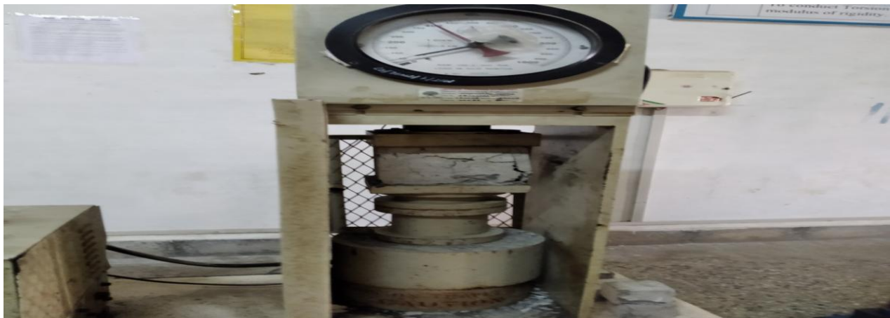
Fig 2.4 Compressive Strength Testing Machine
