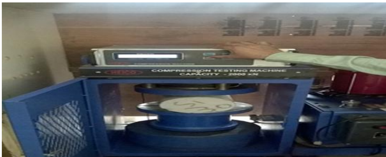
Fig. 2.5 Split Tensile Test machine
