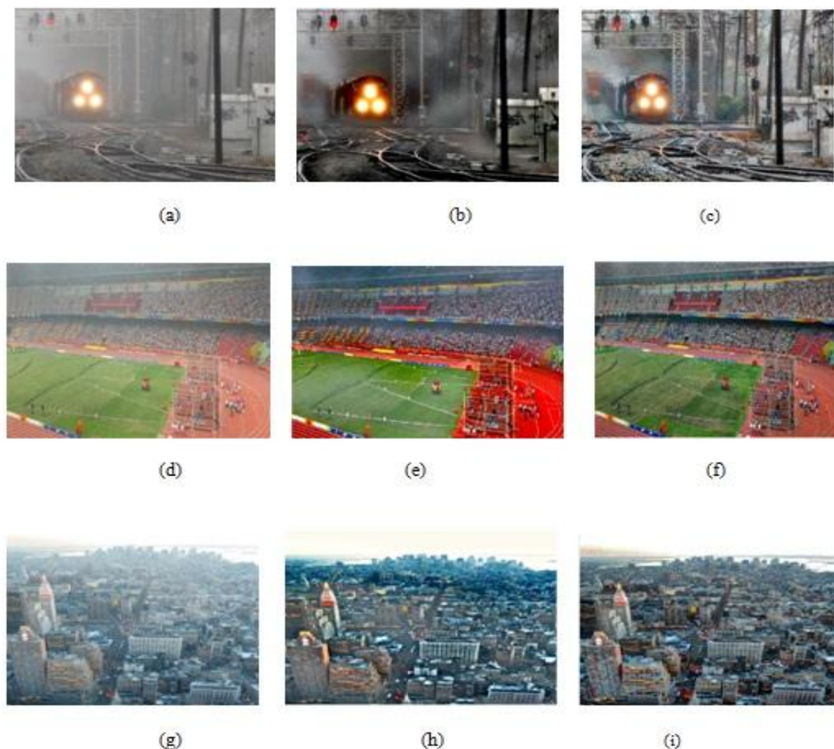
Fig. 5: Original hazy images (a): Train, (d): Ground, (g): City1; previous method [7] results (b), (e), (h); proposed method results (c), (f), (i).
