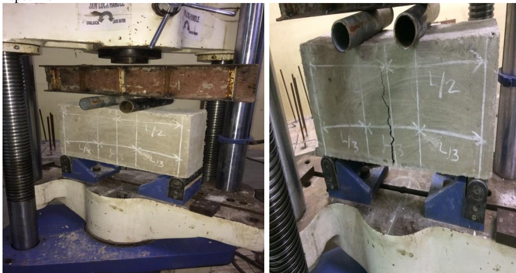
Figure 3 flexural test of block and failure of block
