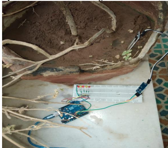
Figure 8: moisture sensor inside pot to sense moisture content
