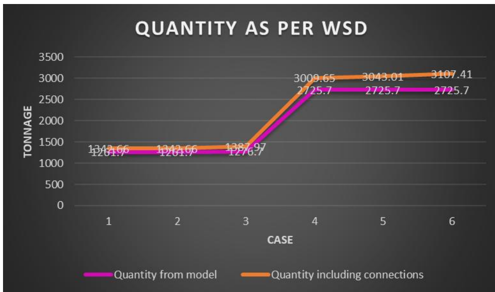
Figure 4 Graph indicating the main steel quantity and quantity including connections for all cases (as per WSD)
