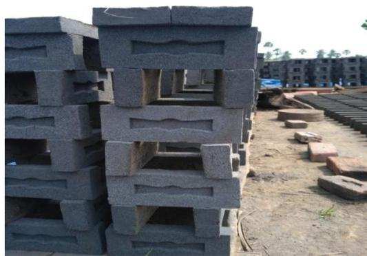
*Fig.4 Drying of Bricks*
