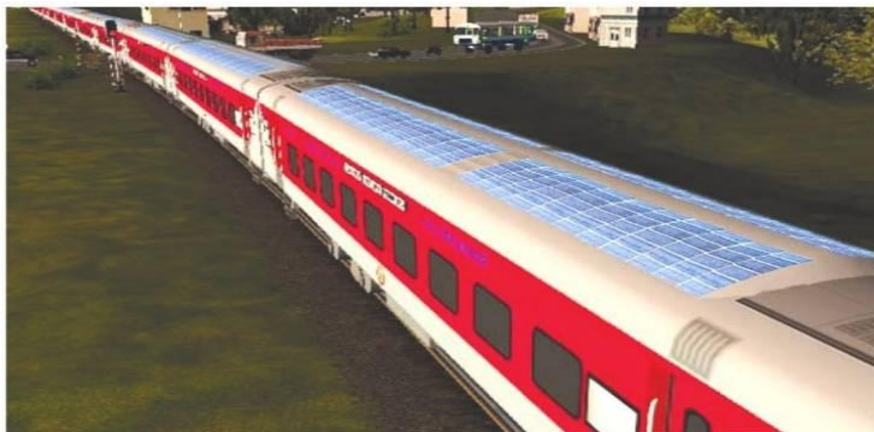
Figure.3 Graphical representation of a LHB coach mounted with solar PV modules
